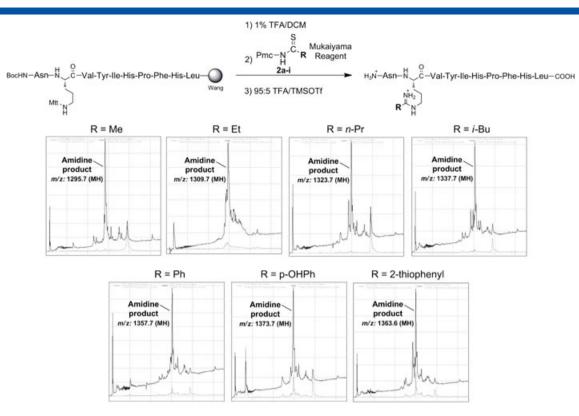
Figure 3. Amidination series on NRVYIHPFHL angiotensin template using Mukaiyama's reagent as the optimized choice of thiophile. A representative series of alkyl-, aryl-, and heterocycle-substituted amidine systems were prepared as Arg headgroup architectural mimics. Crude HPLC chromatograms of each diversified peptide isolate illustrates the generally good purity of peptide product from this methodology.
