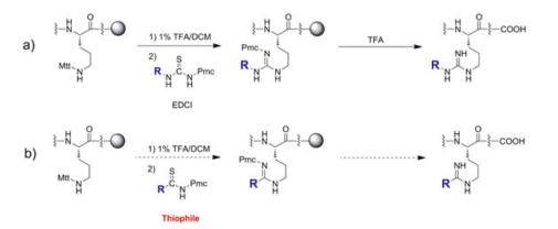
Figure 1. (A) Previously studied synthetic route toward synthesis of on-resin Arg analogs from Orn precursors. (B) Similar proposed synthesis into analogous amidine-based isologs of Arg from Orn precursors.
